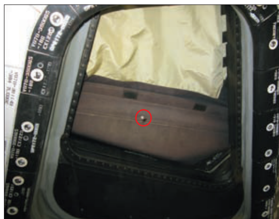
FIGURE 6.1.4 MMOD impact damage to window #6 on space shuttle Endeavour during STS-126 mission in November 2008. The impact damage measures 12.4 mm by 10.3 mm (measured parallel to the glass surface), with a depth of 0.62 mm. According to NASA's Orbital Debris Program Office, this is the largest shuttle window impact ever observed. SOURCE: Courtesy of NASA, from J. Herrin, J. Hyde, E. Christiansen, and D. Lear, STS-126 shuttle Endeavour window impact damage, Orbital Debris Quarterly News 13(2):4, April 2009.
